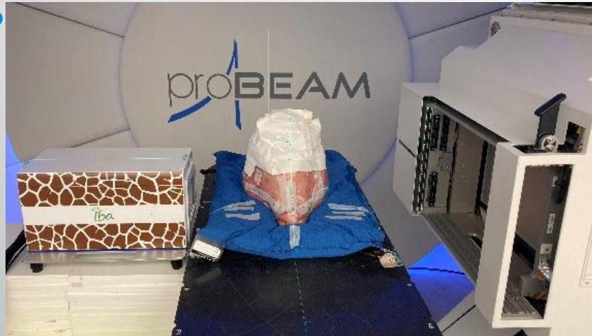
(a) Range measurement setup for pig head
